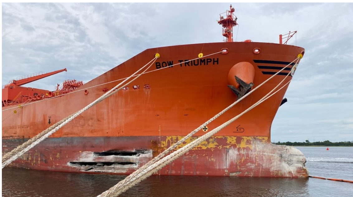
Figure 6. Bow Triumph at the Odfjell Terminal in Charleston on September 8, 2022, showing damage to the vessel's starboard side. (Source: US Coast Guard)
